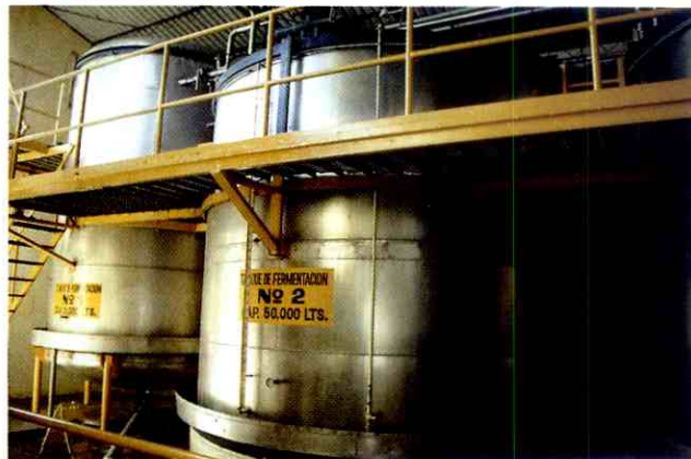
The aguamiel mixed with water ferments naturally because of its sugar content. (Casa Cuervo, Tequila, Jalisco.)
